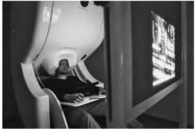
Fig. 12.10 Left: subject wearing a 64-channel (electrode) EEG cap. Right: subject doing a visual stimulation study in an MEG scanner housing 306 sensors.
